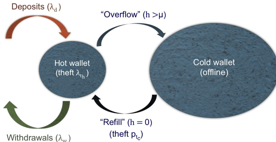
In this study, we analyze the following simple two-wallet configuration (see Fig. 1). Our institution services deposits and withdrawals from a *hot wallet* that is continually connected to the Internet, and suffers theft, which empties the hot wallet, with Poisson rate parameter  $\lambda_{th}$ . For example,  $\lambda_{th} = 0.002$  would
